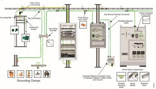
Figure 2-13 Industrial Grounding Network
