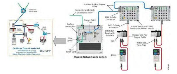
Figure 3-6 Linear Connectivity Deployment Example
