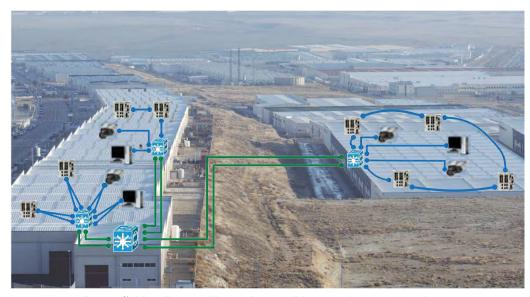
Figure 2-1 Network Overlay on Building Locations
