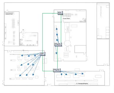
Figure 2-4 Example Use of PNZS and IDFs to Efficiently Distribute Cabling Using a Physical Zone Cabling Architecture
