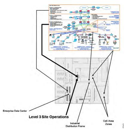
Figure 4-1 Mapping CPwE Logical to Physical
