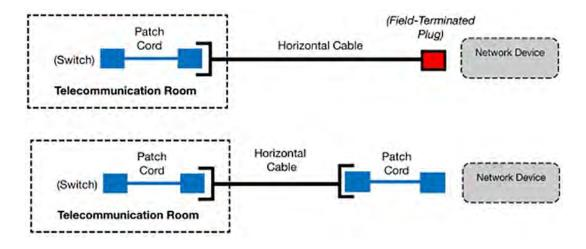
Figure 3-17 Field terminable plug, Field cord
