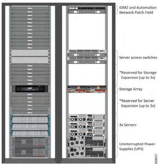
Figure 5-14 The Industrial Data Center from Rockwell Automation—Physical Layout
