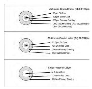
Figure 4-4 Cross-Section of Fiber Construction Types
