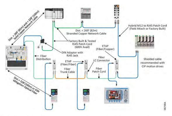
Optical fiber is also used in the Cell/Area Zone. Frequently, Cell/Area Zone installations use IP67-rated connector options. Copper cabling using M12 connectivity (see the following figures) or IP67-rated RJ45 connectivity is applicable in many environments and applications.
