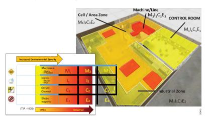
Figure 2-6 Sample Environmental Analysis Using the M.I.C.E. System
