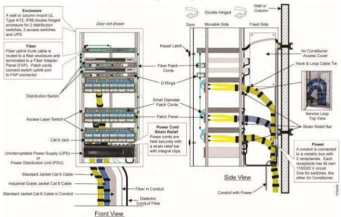
Figure 4-18 Typical IDF Deployment
