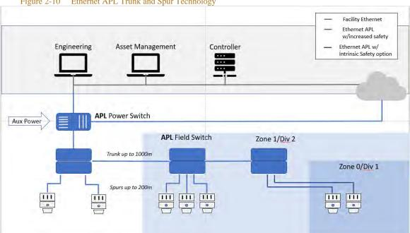
Ethernet-APL (advanced physical layer) is a ruggedized, two-wire, loop-powered Ethernet physical layer that uses 10BASE-T1L plus IEC extensions for installation within the demanding operating conditions and hazardous areas of process plants. It enables a direct connection of field instrumentation to plantwide Ethernet networks in a way that process plants can benefit from a convergence of their OT and IT systems.
