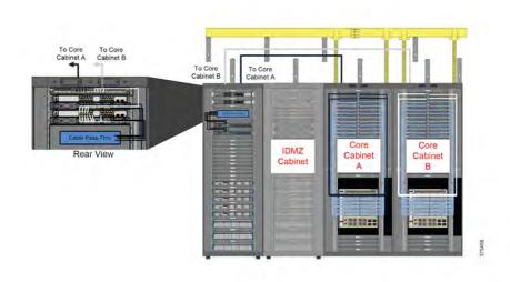
Figure 5-13 Catalyst 9300 Switch to Catalyst 9500 Switch Single Line
