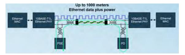
Figure 2-9 Power over data line architecture
