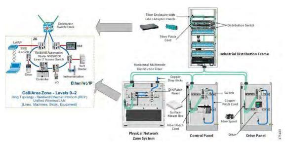
Figure 3-10 Switch-level Ring Topology in the Cell/Area Zone
