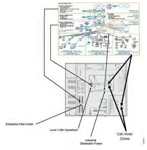
Figure 3-1 CPwE Logical Architecture to Physical Plant/Site
