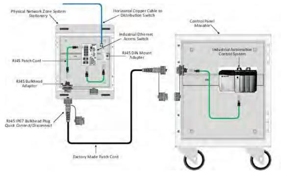
Figure 3-13 Quick Connect Variant 1 Example
